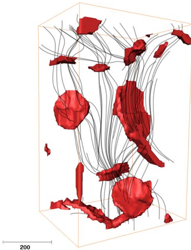
Fig. 4 Predicted Stokes flow (from top to bottom face) through a bioactive glass scaffold with only the flow and interconnects visualized. Scale bar in microns
